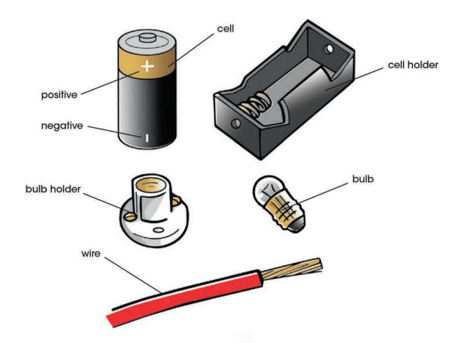
A cell pushes electricity around a **circuit**. It has a positive (+) side and a negative (-) side. The **bulb** lights up when electricity goes through it. The wire is used as a **connector**.
